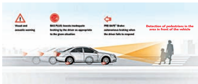
▲ Fig. 10 Pre-safe brake – developed and confirmed for sedans – now in trucks (Source: Daimler AG, Stuttgart, Germany).
