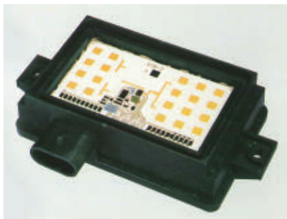
▲ Fig. 5 24 GHz SDS system built by HE Microwave, 1995 (Source: HE Microwave publication, IEEE MTT-S, 1995, San Francisco, USA).
