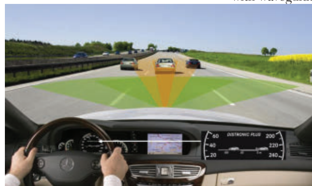
▲ Fig. 4 Antenna configuration schematic of DISTRONIC PLUS, where orange is a 77 GHz LRR-sensor and green is a 24 GHz SRR-sensor (Source: Daimler AG, Stuttgart, Germany).
