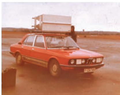
▲ Fig. 1 10 GHz automotive radar system built by VDO in the early 1970s (Source: private collection of the author).
