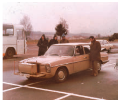
▲ Fig. 2 16 GHz automotive radar system built by Standard Electric Lorenz (SEL) in 1975 (Source: private collection of the author).
