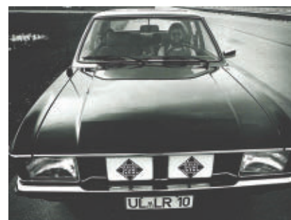
▲ Fig. 3 35 GHz automotive radar system built by AEG-Telefunken in 1974 (Source: private collection of the author).
